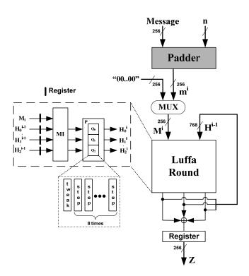
Fig. 1. Hardware implementation of the Luffa hash function
